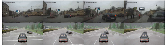
Figure 4: Vehicle Cutting In with Pedestrian Crossing Scenario : in the original dash camera video (top row), the vehicle on the right performs an emergency lane change to the left due to a jaywalking pedestrian in red. In the generated scenario (bottom row) produced by our framework, the vehicle on the right exhibited a similar lane change behavior to the left to avoid a jaywalking pedestrian.
