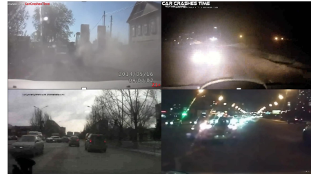
Figure 9: Scenarios from the Car Crash Dataset where our current framework cannot handle due to heavy traffic with multiple cars or compromised lighting environmental conditions at night
