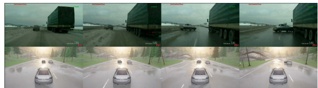
Figure 6: Vehicle Spin Scenario : in the original dash camera video (top row), the vehicle in front of the ego first spins to the left and then collided into the right vehicle. In the generated scenario (bottom row) produced by our framework, the front vehicle exhibited a similar spin and collision behavior
